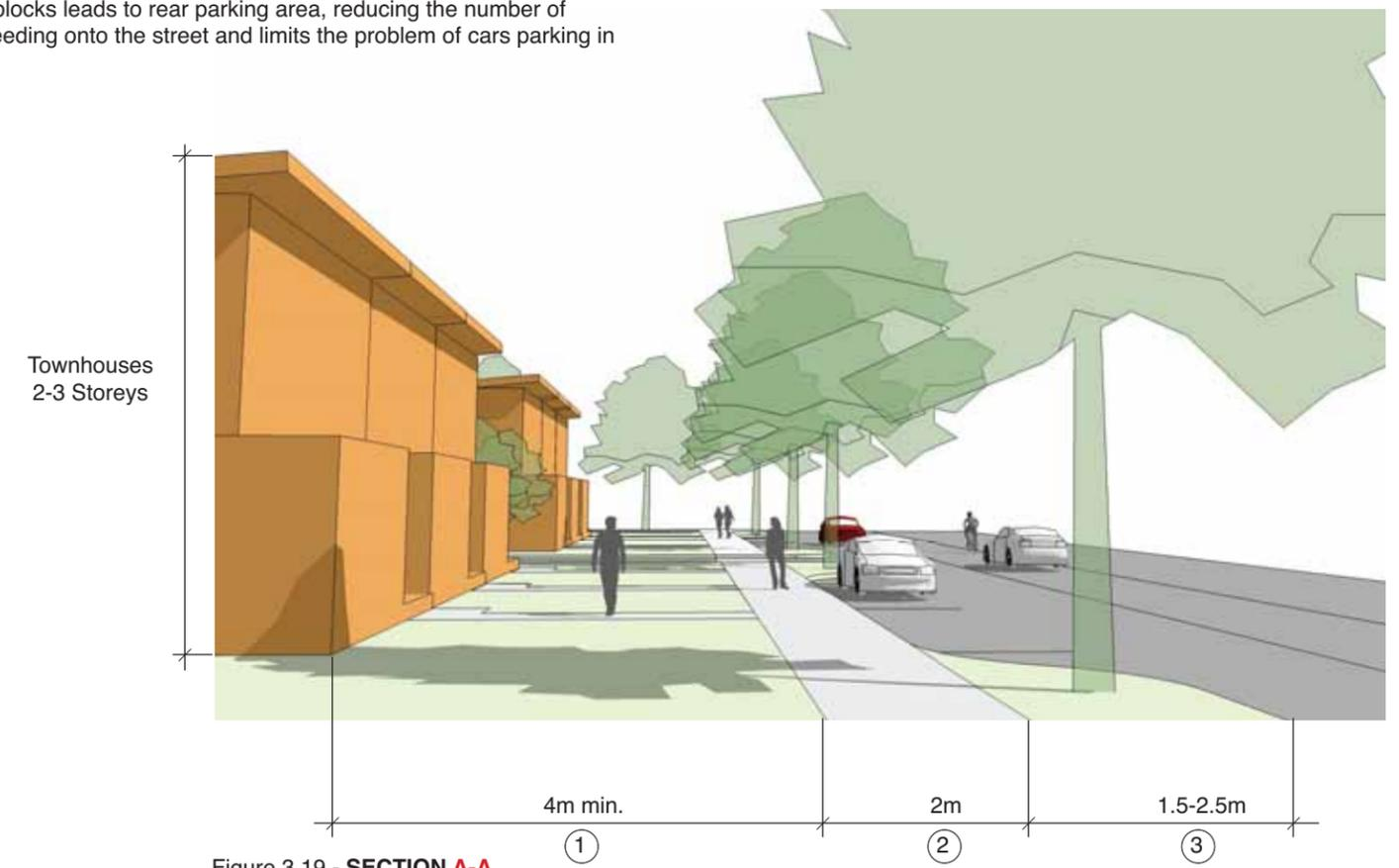
Figure 3.19 - SECTION A-A
