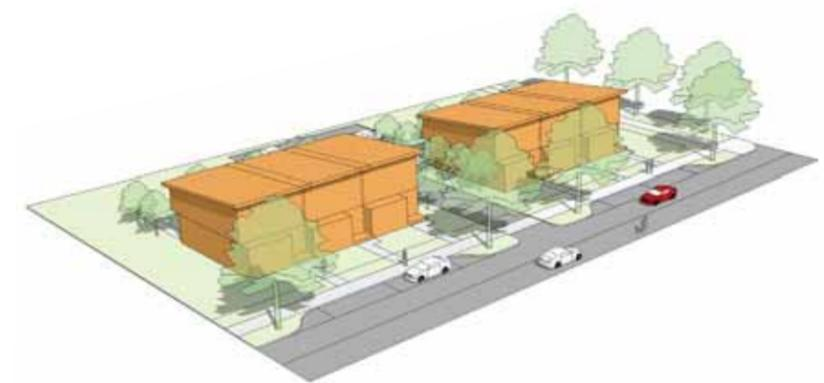
Figure 3.17 - Massing of a Typical Townhouse. Shared driveway between townhouse blocks leads to rear parking area, reducing the number of driveways feeding onto the street and limits the problem of cars parking in front yards.
