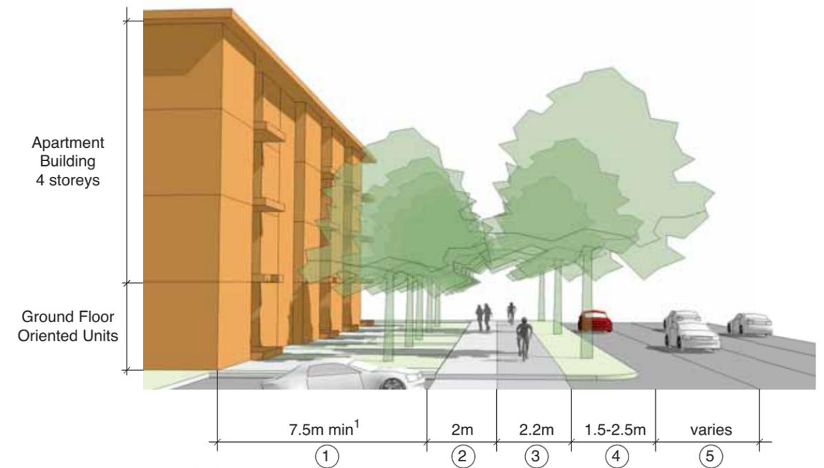
Figure 3.14 - SECTION A-A
